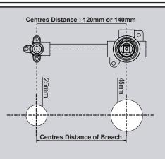
3 Check centres distance of the breach assembly for 120mm or 140mm size for 120mm or 140mm size. Mark centre line according to measured result.
