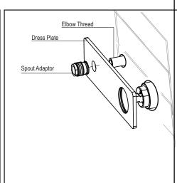
Remove the protective cover from the mixer. Apply Teflon tape to Elbow Thread. Gently, push the dress plate to position. Screw Spout Adaptor to Elbow Thread with a spanner or Allen Key.
