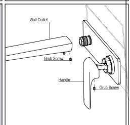
**5** Push Wall Outlet to the spout adaptor and fasten Grub Screws to secure Wall Outlet. Fit handle to position and tighten grub screw to secure handle.
