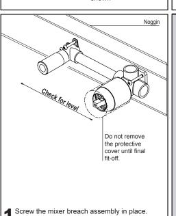
Screw the mixer breach assembly in place. CHECK OUTLET AND MIXER ARE LEVEL.
